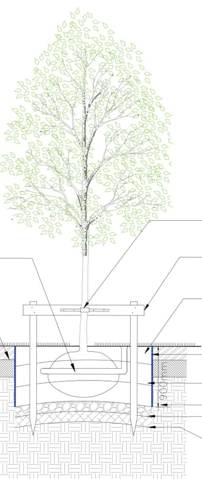
The tree is to be secured to the cross-bar using 1no. rubber felt back block secured with rubber belting tie. Rubber belting tie fixed with 4no. clout nails. Ties are to be secured so as to allow for movement but prevent damage to the trunk.
